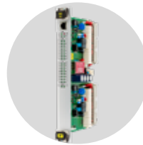
Netcon GW502 CPU of Netcon 500 Substation RTU
