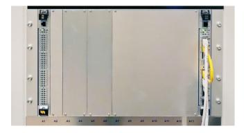
For each of the substations, one Netcon 500 RTU was put into operation to enable the communications between the substation IEDs and the central HMI. As a modular hardware platform that supports 50+ communication protocols, the Netcon 500 is well prepared for forthcoming changes, should they be required, including various makes of IEDs.
